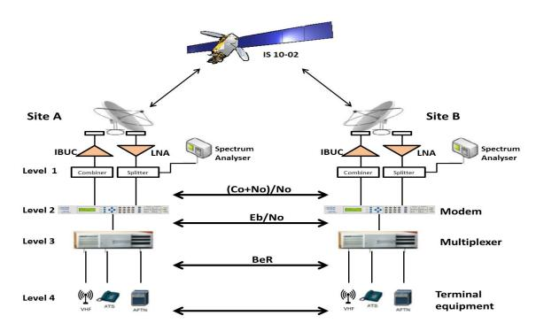
**Figure 2:** Four level VSAT performance monitoring approach between Site A and Site B.
