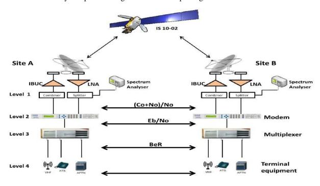
Figure 1: Four level performance monitoring approach between Site A and Site B.
